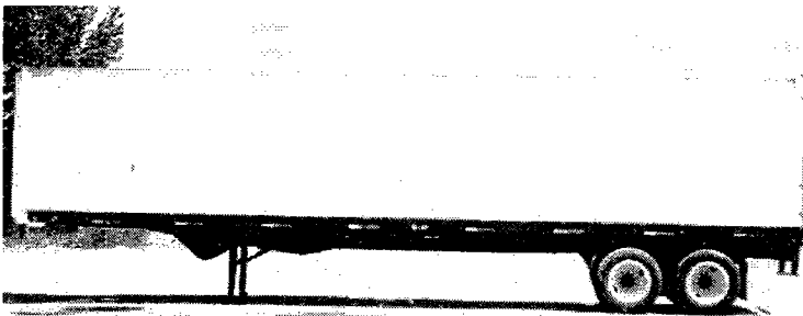
Figure 6. Semi trailers are the cargo carrying units of combination vehicles. Note the retro reflective tape down the side of the trailer to prevent under-ride collisions. A semi trailer is considered a "vehicle."
